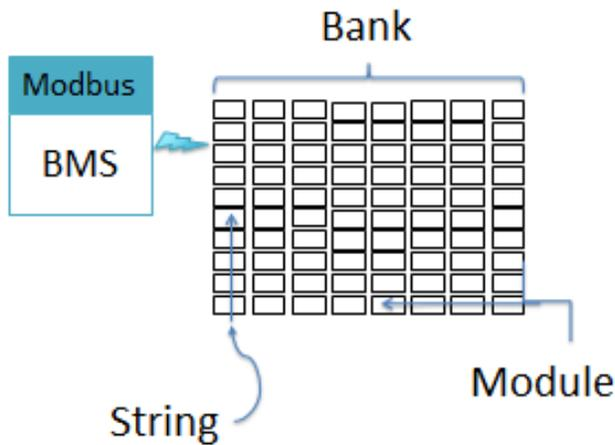
The battery management system (BMS) communicates with battery strings and modules, and surfaces aggregate data. Different vendors expose many common attributes: state of charge, current limits, temperature alarms, etc. Many BMS implementations use Modbus today, and the SunSpec Energy Storage Specification defines standardized sets of software interface to these registers for compatibility and plug-and-play operation.
