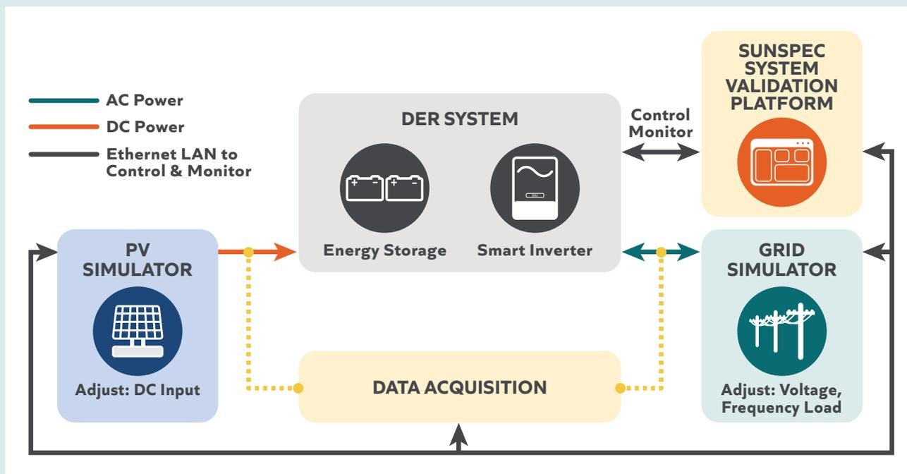
Figure 1. SunSpec System Validation Platform (SunSpec SVP)
