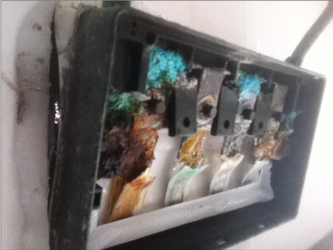
Figure 13. Manual inspection and testing requires opening NEMA-rated enclosures. The integrity of any enclosure seal must be restored after opening to avoid moisture damage as in this module junction box. (photo by Andy Walker)
