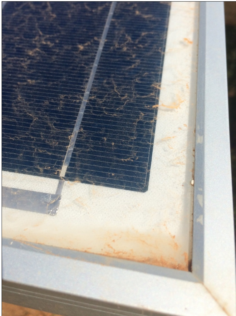
Figure 6. Module soiling can often be traced to a source, such as construction-site dust shown here resulting in about 5% loss. (photo by Andy Walker)
