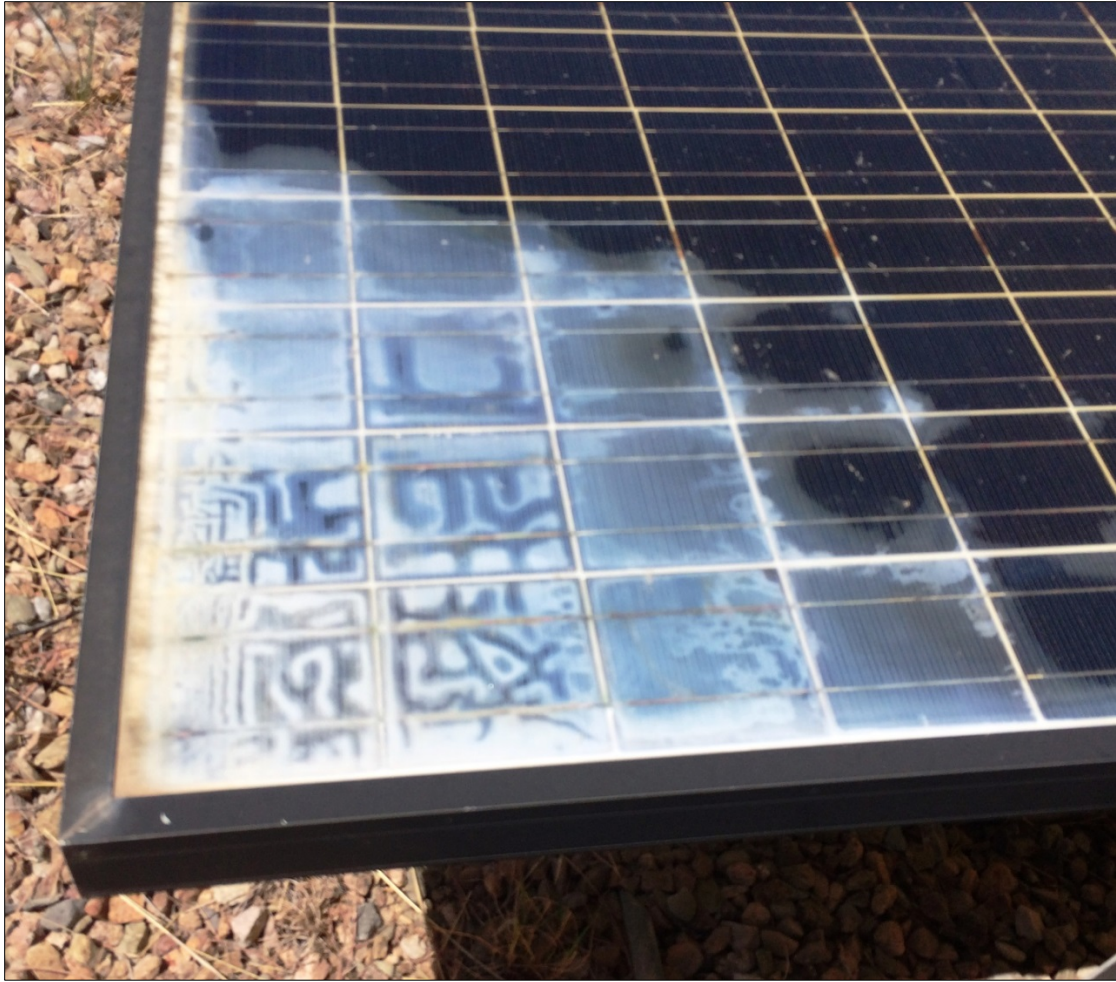
Figure 9. Failure in materials and workmanship, such as encapsulant of this module, are often covered by “product warranty.” (photo by Andy Walker)
